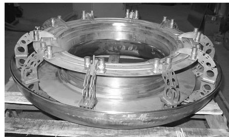
Fig. 4. Support frames adjusted to the dummy coil form and to the lower half-vessel. The top of each frame has two cylinders with Inconel 625 springs providing 450 kg compression to the coil inside the helium vessel after the final closure.
