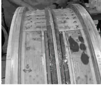
Fig. 3. A Nomex string is wet wound above the insulated joint. G10 ramps, long side arches and side plates are installed for joint support.
