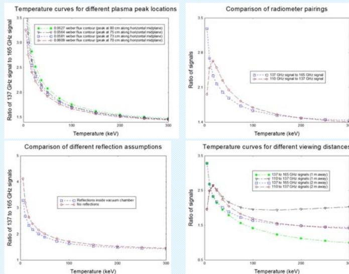
Fig. 1: Optimal temperature curves are steep because it is seen that a slight change in the position of the plasma peak significantly affects the apparent hot electron temperature. These curves were generated assuming the radiometers viewed the plasma vertically.
