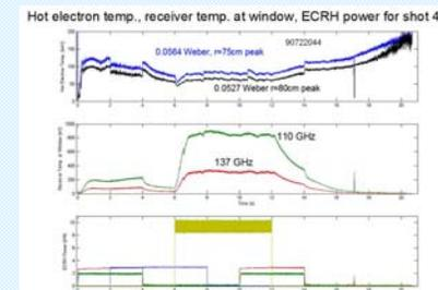
Fig. 3: The curve for peak location at 80 cm along the midplane is almost continuous with the curve for the 75 cm peak location around 2 seconds into the shot. The modeling done for this study could be used to track the movement of the plasma peak during experiments.
