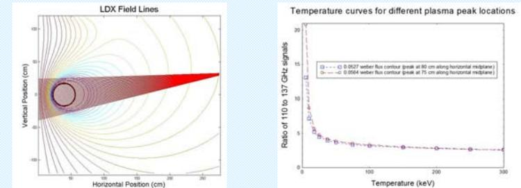
Fig. 2: When the plasma is viewed along the horizontal midplane from the chamber wall, the beam diverges above and below the F-coil and sees into the high field region. The emission from this region dominates the detected emission. From this viewing position, the position of the plasma peak has a less significant effect on the apparent hot electron temperature.
